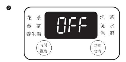
After the plug is inserted into the power socket, "OFF" will appear on the display screen and there will be a "BEEP", which suggests that the product is standby.
