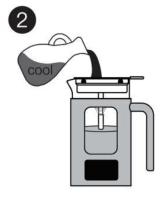
Add water into the kettle and make sure the clear water in it is between the lowest mark(200ml) and the highest mark(600ml).
