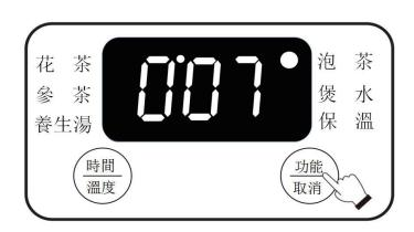
Press "Function/Cancel" gently and choose the "Brew Tea" program. The program indicator will flicker. The default time is 7 minutes and the default operation temperature is 100  $^{\circ}$ C and cannot be adjusted. Press "Timer/Temperature" gently to adjust the operation time of heating (5-60 minutes): short press the button to increase by 5 minutes each press, or long press it to increase by 10 minutes each press. The adjustment can be cyclic.
